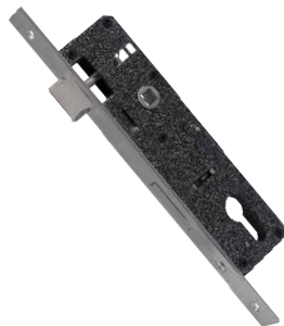
Mortise Lock - 30 mm Special Mortise lock cylinder for metal & wooden Doors Reversible Latch bolt & dead bolt by 1 turn Finish : Satin Stainless Steel Centre : 30 x 85
